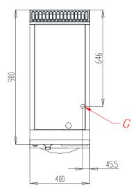
G gas connection | E electric connection | CW cold water connection | HW hot water connection | SW soft cold water connection | D drain
